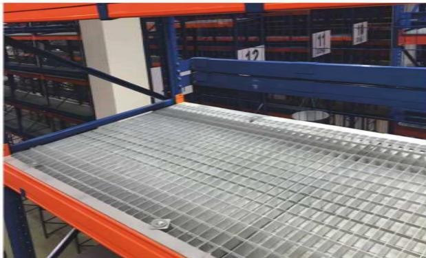
**A characteristic feature of the product is the framing**, which helps to support and stabilize the grating shelves placed on or between the load beams of the rack. The framing can take the form of a flat bar (optionally an angle bar or C-Channel) with a height greater than the height of the grating.
